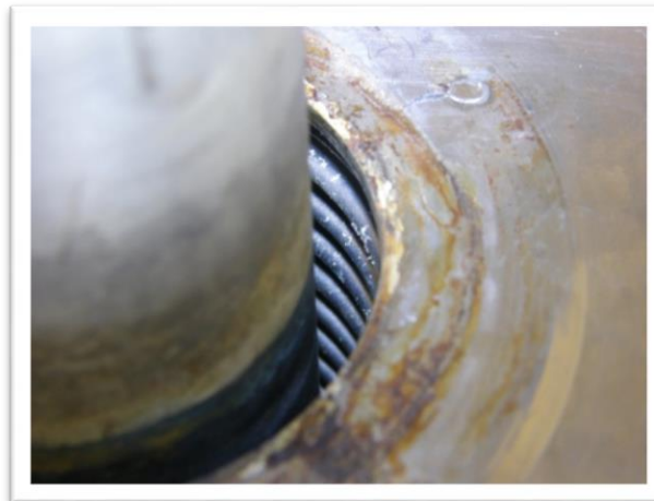
Image 2 - Saltwater contamination on bellows.
