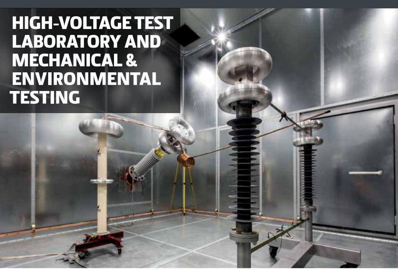
Available for testing or certification of your equipment, our high-voltage laboratory is equipped with the specialized test equipment and measuring instrumentation to evaluate and certify low- and medium-voltage electrical equipment such as circuit breakers, switchgear, insulators, transformers, power cables, arresters, capacitors, pole line hardware, bucket trucks, vacuum interrupters. Additionally, we have the capability of performing a wide variety of mechanical and environmental tests.
